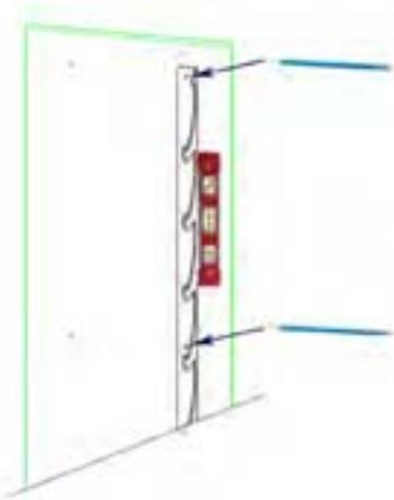
4) Drill with a 5/16" tip = 8 mm in The marked points, insert the PVC plugs.
