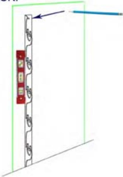
2) Hold the level horizontal, place it on the upper mark already made in the hole, make a second mark to the right, at a distance of 6 1/2" = 170 mm.
